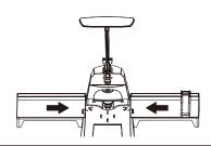
B-4. Adjust the paper guide according to your requirement. Hold the paper securely with one hand and pull down on the handle to complete a cut.
